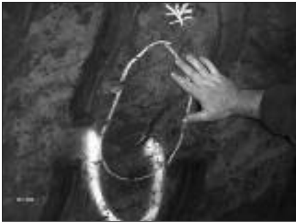
Fig. 23 Deep tread rock cut – If left unattended will cause cut separation or cut through.
