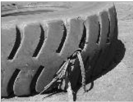
Fig. 15. Rapid air loss like this occurs frequently when tires are overinflated and suffer an impact.
