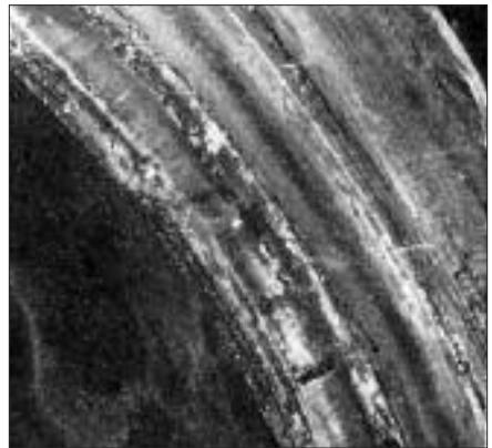
Fig. 22. Heal damage due to burned bead.
