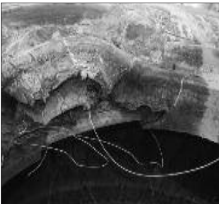
Fig. 21. Rupture resulted from burned bead.
